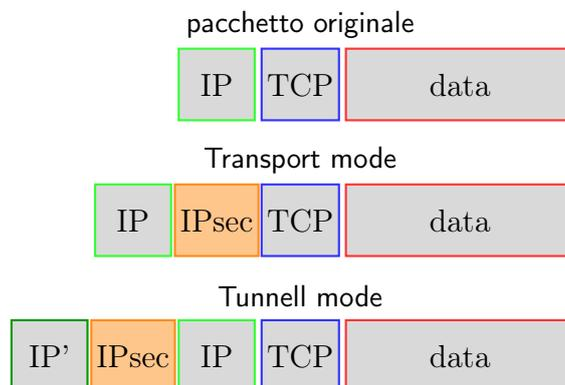
Figura 32: schema incapsulamento IPsec
